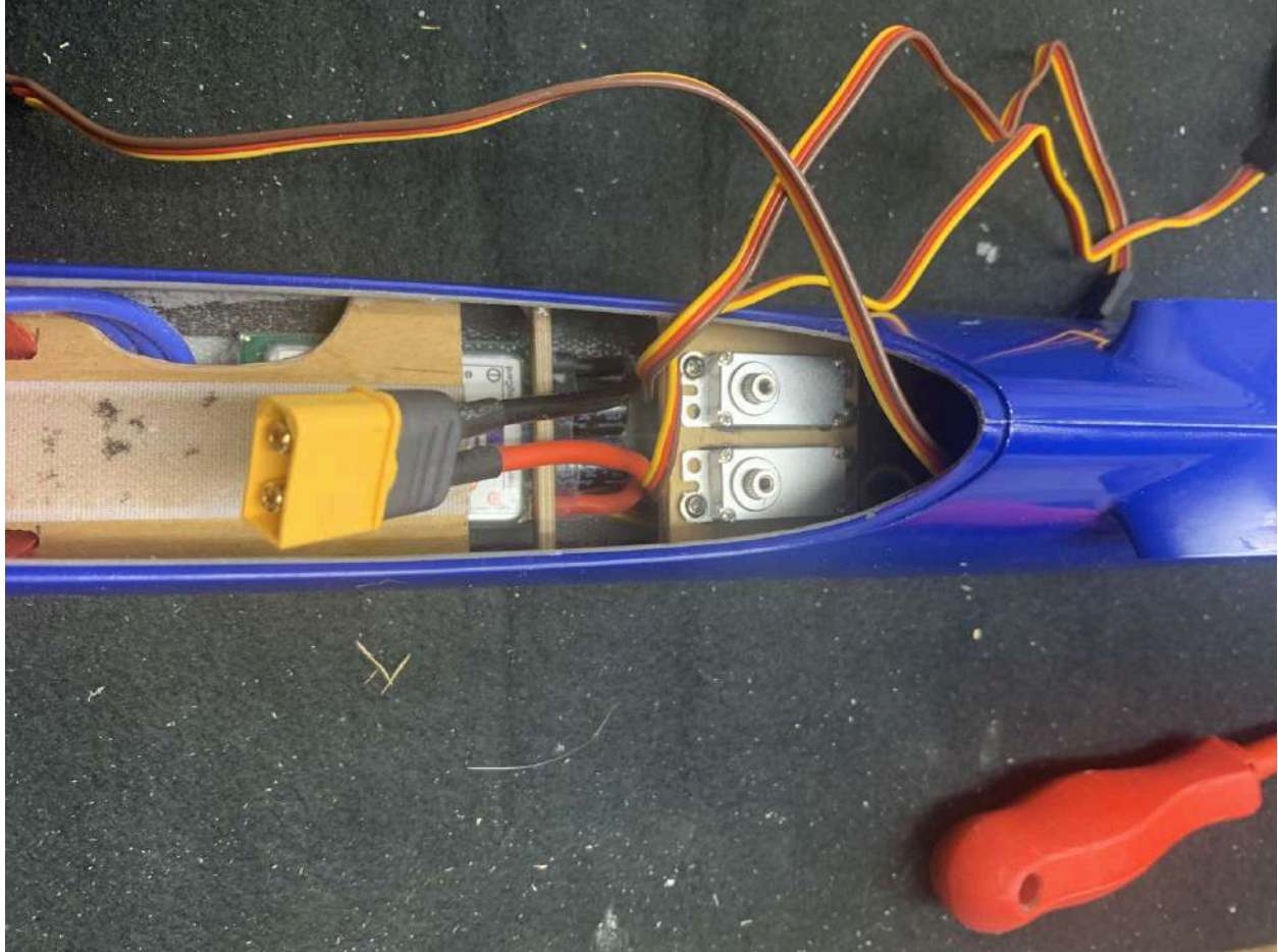
Rudder and elevator servos behind the battery
