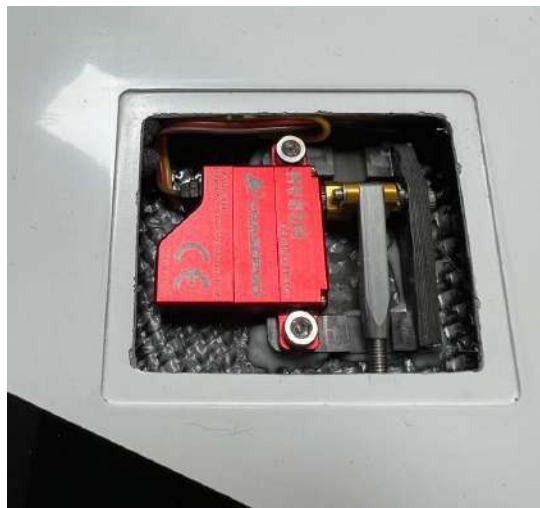
The wing servos built in the pockets.
