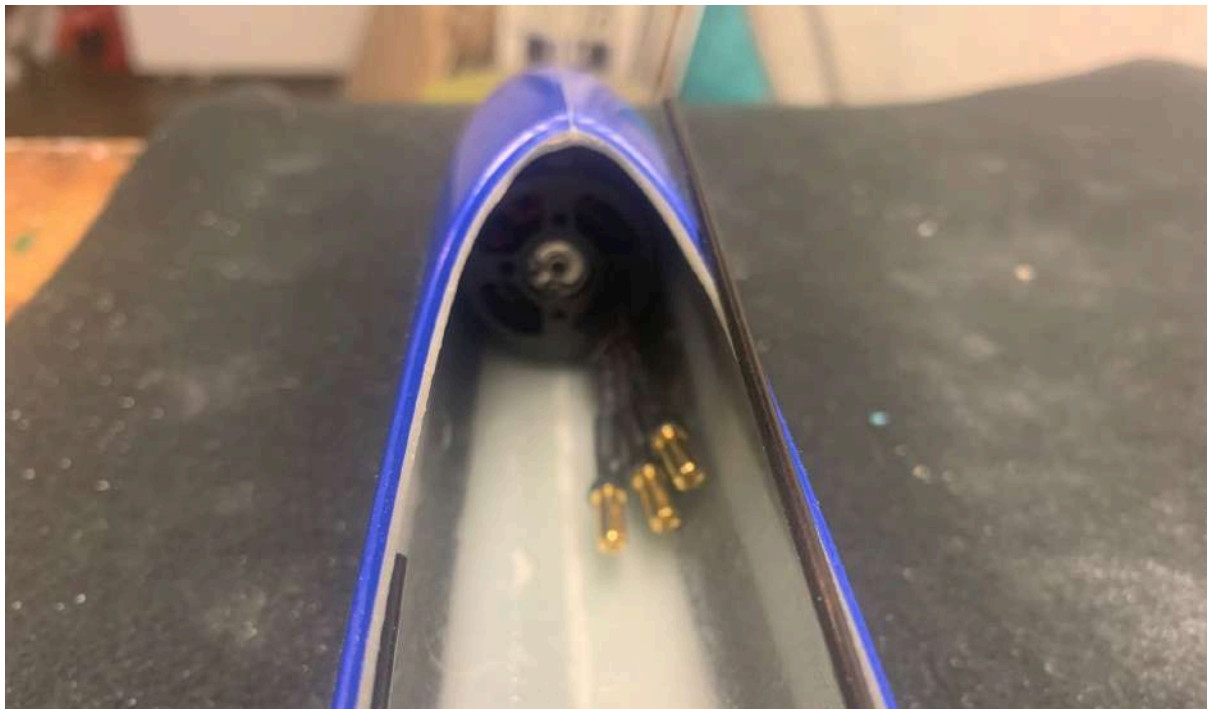
Motor mounted in fuselage
