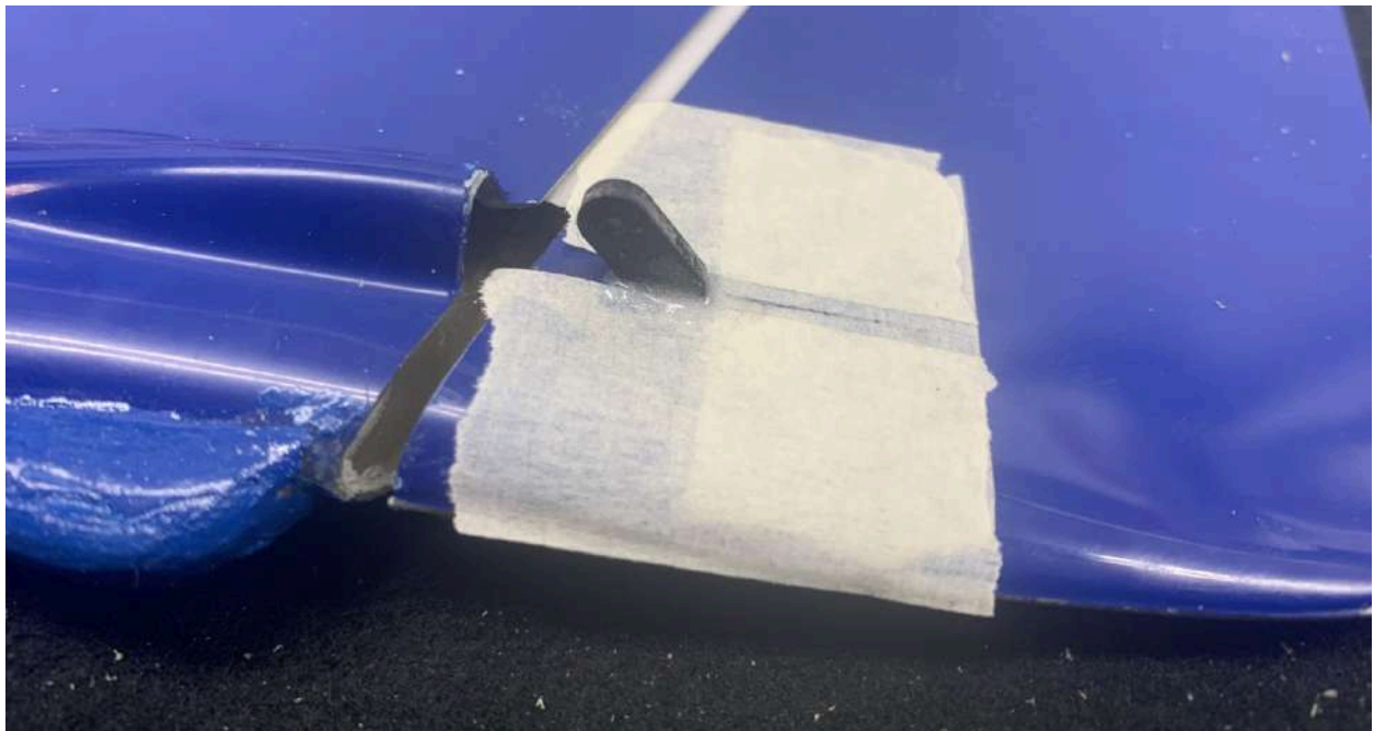
Gluing the rudder horn.
