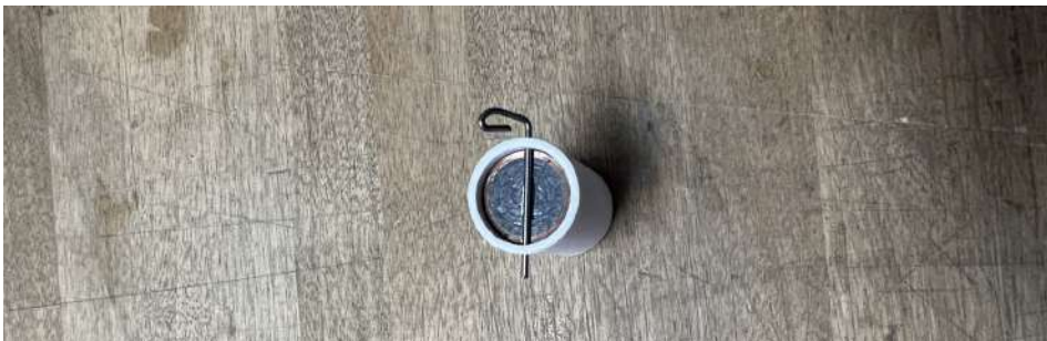
50 gram as counterweight in the fuselage
