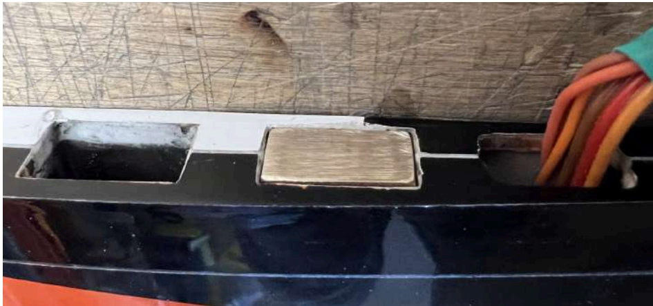
Ballast inserted in the wing
