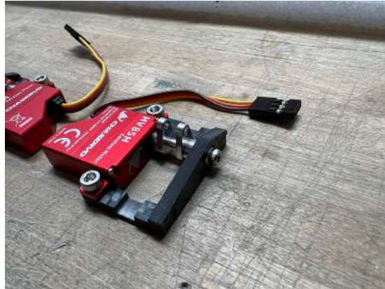
Servo with counter-bearing
