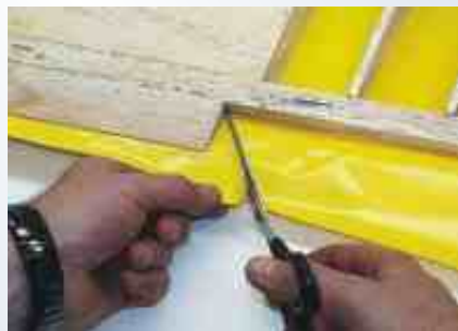
Fig. 12a For inside corners, first slit 45°.
