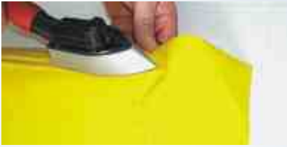
Fig. 9 / 9a Gradually work around curves
