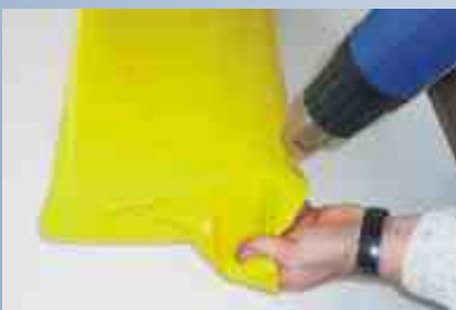
Fig. 11a-d Covering of the wing tip
