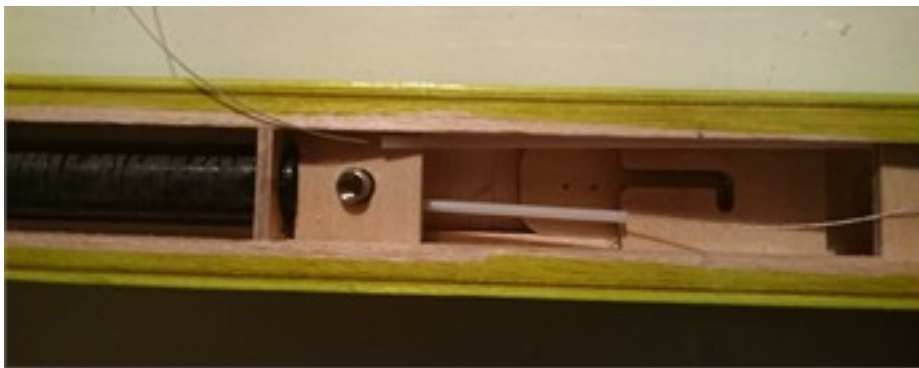
The rope plastic tubes be laid from the servo department to about 1cm into the tail boom. Inside the tail boom the ropes lie free without the plastic cable housing.
