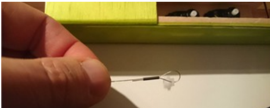
Rope with crimp connected to the Servo horn.
