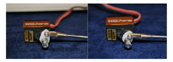
To prevent the pushrod fouling the shafts the arms are set at 2 clicks off centre for the ailerons towards the TE and one click for the flaps.
