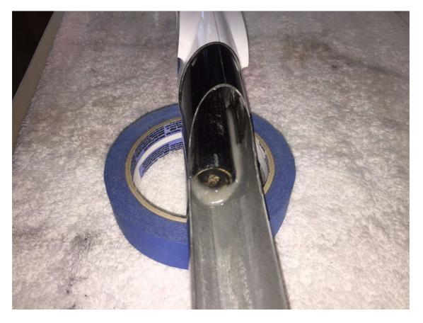
Finally, fit the radio tray, it should be approximately 12mm below the edge of the fuselage at the centre of the canopy area. With a methodical working you will be able to do quite neatly but do ensure a good joint to the ballast tube and fuse with the tray. It won't be doing much if not bonded properly.
