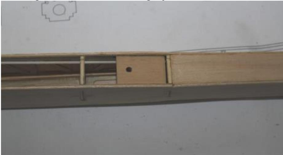
Now the pushrod housings can be glued to the fuse bulkheads. Ensure the housings are as straight as possible. It is recommended that the steel pushrods be inserted to help straighten them. A slot still has to be cut into the side wall for the rudder pushrod housing.
