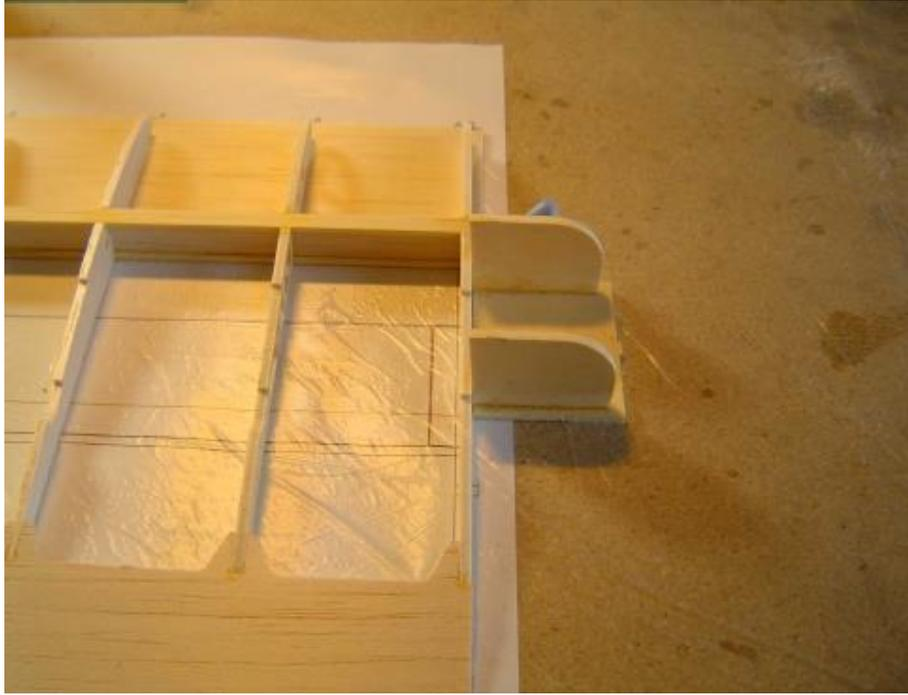
Roughen and thoroughly clean aluminum wing joiner tubes. Slide aluminum tube into ribs A-9 and A-8. Align at 90 ° to end rib. Gap between tube and spar webbing will be filled in with scrap 1.5mm plywood. Coat ply filler, Al tube, and spar webbing with epoxy and assemble. Picture shows top spar in place, but do this step before top spar is glued in so the ply filler can be inserted.
