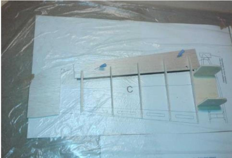
Make a false leading edge from 2mm scrap balsa. Shape top edge for upper planking. Cut top planking so it will extend over the wing tip. Glue on upper planking.
