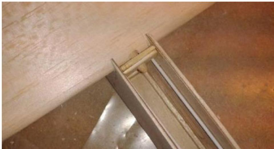
The wing retaining piece in the fuselage.
