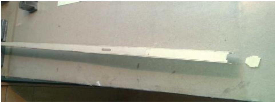
Finally, the adjustable tow hook and the balsa nose are glued with white glue. To accommodate trim weight, the nose can be slightly hollowed.
