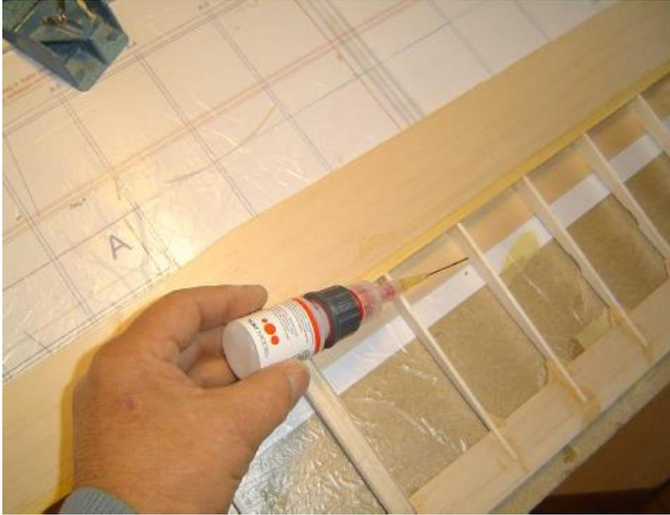
Now, through the gap between the strip on the nose and the upper planking, glue the upper planking to the ribs. Here it is advisable to use thin needles and take advantage of the fluidity of the superglue. Planking needs through the gap from the front are glued to the ribs.
