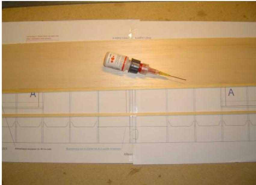
The ribs are cut and sanded to fit on the pine spar. The 3mm balsa spar webbing is also prepared.
