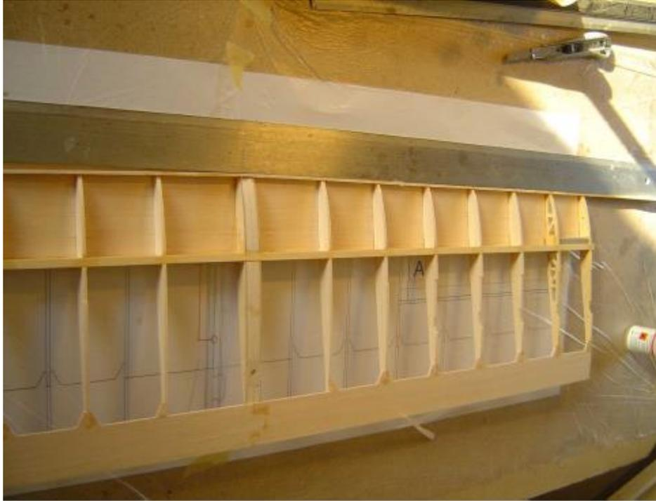
Now a strip of balsa 2 mm is cut from scrap balsa sheet and glued to the front of the ribs. Take a long ruler or a straight bar as a sanding block to make the front edge straight.
