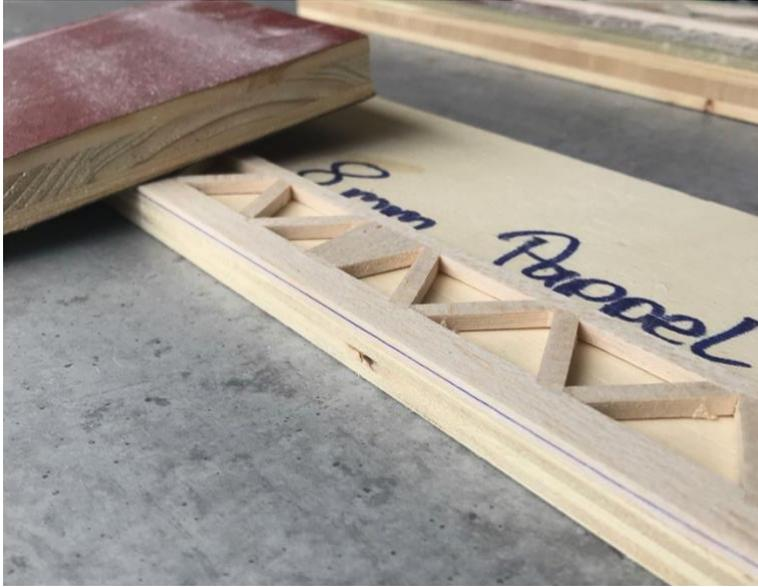
The sanding batten on the trailing edge of the tail unit and the Edge of the table. So grind we the trailing edge down to ours Auxiliary line from both sides (approx.1mm) pointed. In contrast to the trailing edge, the we just sharpened it to a point we grind them The leading edge of the tail units is round. For this we grind on both Sides of the leading edge of the Tail unit a 45 ° phase, which is approx. a third of the wood thickness occupies. This phase helps us again, an even
