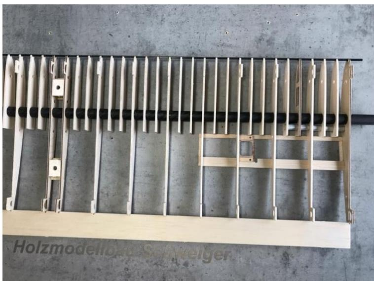
The component A2V is located on the 8mm balsa board and is placed under the plywood part A1V glued and engraved flush. Tip: a drill with the Diameter of 5mm through the balsa blocks A2V at Glue stuck so that the Holes exactly one above the other lie. The upper planking (1.5mm Balsa) is attached to the leading edge adjusted and at the end about 2-3mm shortened. The shortened end the planking is the
