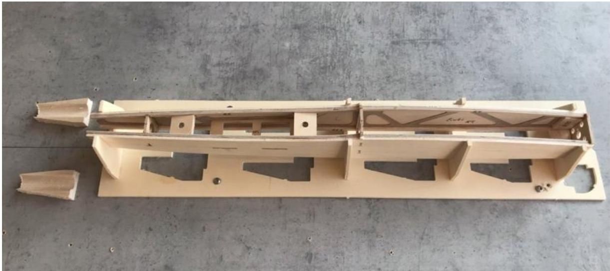
**Tip:** We screw the fuselage slipway to our building board!
