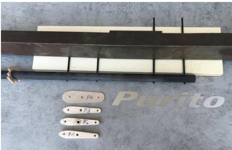
The pylon part P1 can now be fitted and glued in place. For component P2, make sure that the M3 nut points upwards. Attach and glue the P2 and P3 components as well. Only part P4 must not be glued yet, because this will be done later with the elevator. The carbon rods that protrude from the top of the elevator pylon should be shortened to 4.5mm (so that they no longer protrude when the elevator is screwed on)
