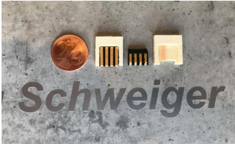
We use for that Power connection to the hull a 5-pole spring contact. This is also with us as Accessories available. Like on that Can be seen in this picture Milled accessories too Plywood parts that contain the Spring cotter precisely fits into the Wing recording takes up. For this execution is Experience in soldering required
