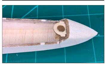
Glue the front magnetic catch into the nose block. The precut slots in the nose block determine the angle for the catch.
