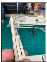
To save the skills required of building a ship in a bottle now is the time to put the PTFE elevator tube into place. This slides through the rear slot is TS2 and through one of the holes in F3. The tube must not be glued at this stage as it may need to the moved once the fin is built.
