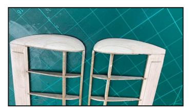
Sand the wing tips and trailing edge to shape. The actual section applied to the wing tips really does not matter and is one of personal taste. An approximate shape is shown on the plan. The Trailing edge of the wing should be sanded so the rear is approximately 1mm thick. Again as example is shown of the wing plan.
