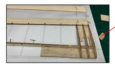
Pin down the trailing edge sheet and add the 3 central wing ribs R1,R2 and R3. Please note that R1 should be glued at an Angle for the dihedral. Use the jig provided to obtain this angle. You can use PVA, CA, Balsa Cement for all of the wood to wood joints on the Micro Runt, we use Deluxe Materials superhatic adhesive for most of out builds. R2 gets cut away for the servo after the top sheeting is added
