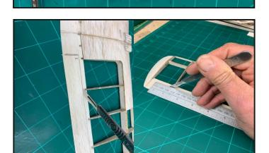
The ailerons can now be cut free from the wing. You have the option of top hinging of centre hinging. Shape the Leading edge of the aileron to suit. We strongly recommend top hinging as it is very important to have a sealed hinge line.
